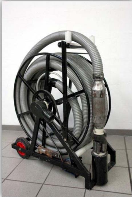
InTube Cleaner principle: It consists of an air-driven motor; responsible for the rotation of a head with steel brushes for cleaning the tubes and at the same time to drive the vertical movement on the tubes for optimum contamination removal such as dust, carbon deposit and scale.
