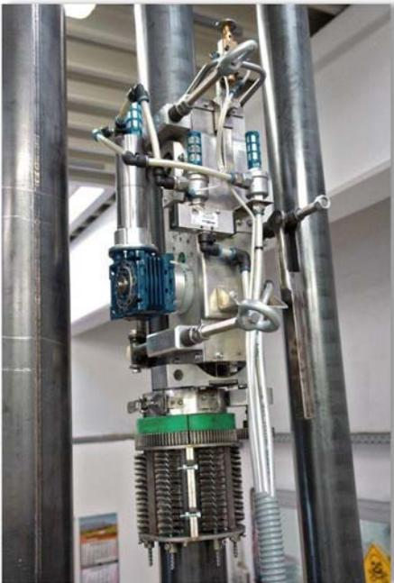
OutTube Cleaner principle: It consists of two air-driven motors; responsible for the rotation of a head with steel brushes for cleaning the tubes and to drive the vertical movement on the tubes for optimum contamination removal such as dust, carbon deposit and scale. The OutTube Cleaner is also equipped with an automatic limit switch on the upper part of the machine in order to drive down the unit upon reaching the complete height of the tube.
