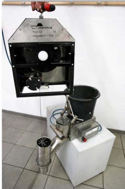
UNIDENSE® technology is used for loading of all common catalyst types and sizes. Reformer tube designs with varying internal diameter, narrow or wide top section, have successively been loaded.
